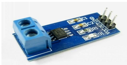
Fig 5.4: ACS 712 current sensor
